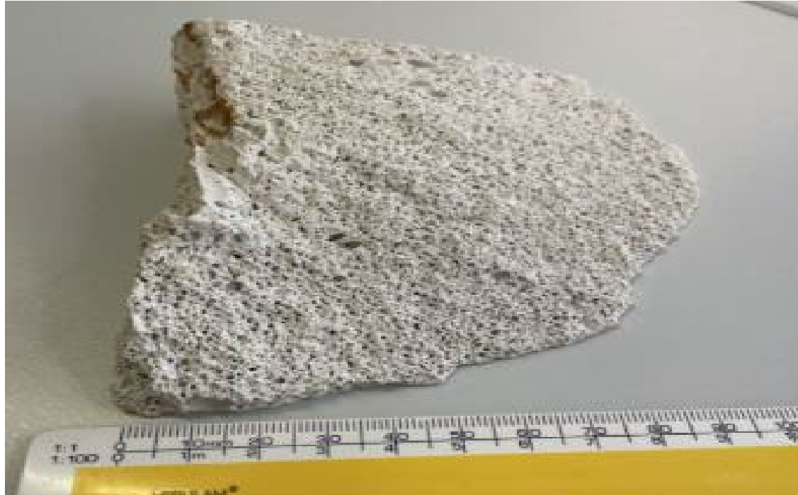
Figure 2: A fragment of RAAC showing its 'bubbly' appearance
