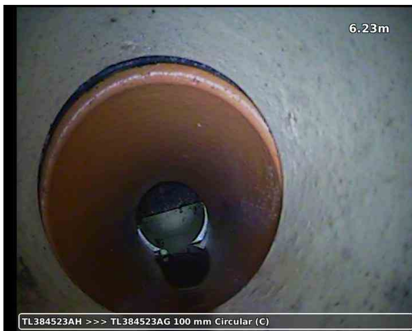
20210617-184209-snap0004.jpg, 00:01:12, 6.23 m Joint displaced, medium
