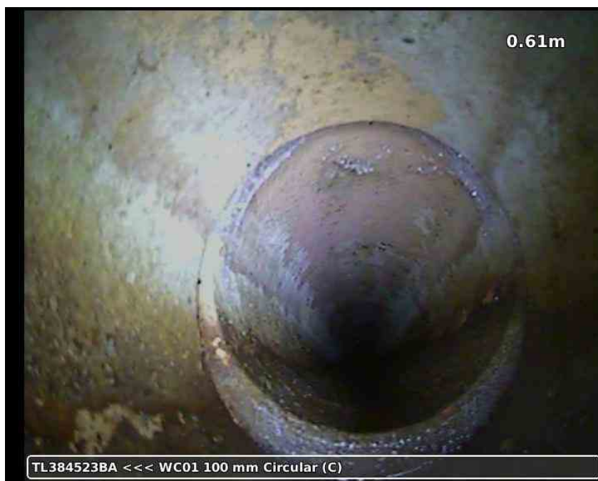
20210617-164432-snap0006.jpg, 00:00:45, 0.61 m Joint displaced, 10 mm displacement
