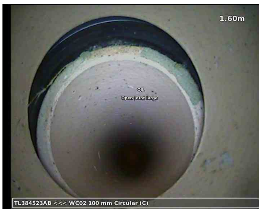
20210617-165855-snap0004.jpg, 00:00:40, 1.60 m Joint displaced, 20 mm displacement
