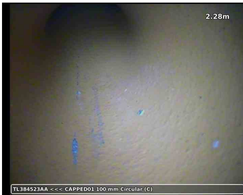
20210617-161651-snap0003.jpg, 00:00:52, 2.28 m Finish node type, other special chamber, reference number: CAPPED01, Internal rest bend CAPPED OFF
